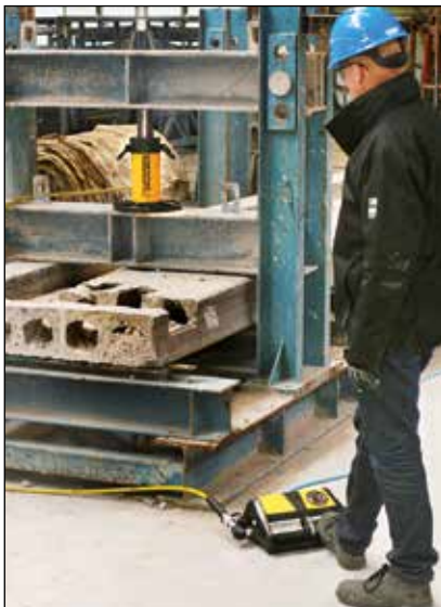
◀ SCR-Series Cylinder-Pump Set with XA11G used for concrete testing.
