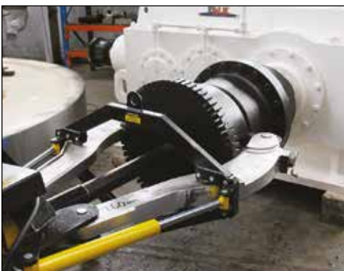
◀ The EPH-1002A quickly and easily removes this drive coupler from its shaft.
